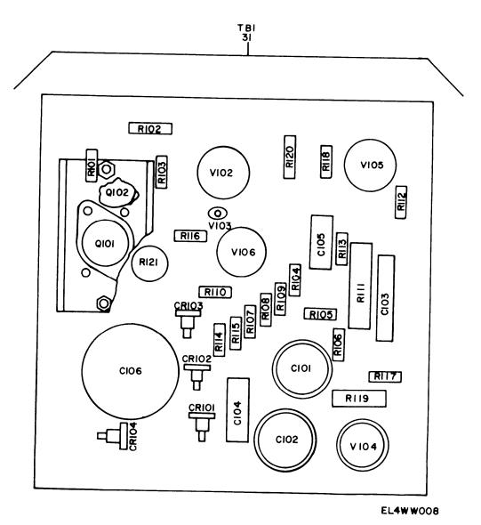
Figure 3. Voltmeter, Electronic, ME-161A/U, Circuit Board Assembly 801B-523 (Sheet 1 of 2).
