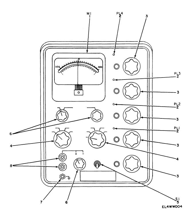
Figure 2. Voltmeter, Electronic, ME-161A/U, Panel Assembly, Front View.
