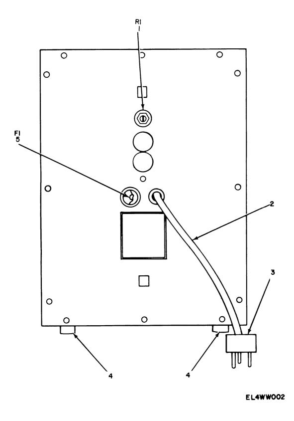
Figure 1. Voltmeter, Electronic ME-161A/U, Rear View.
